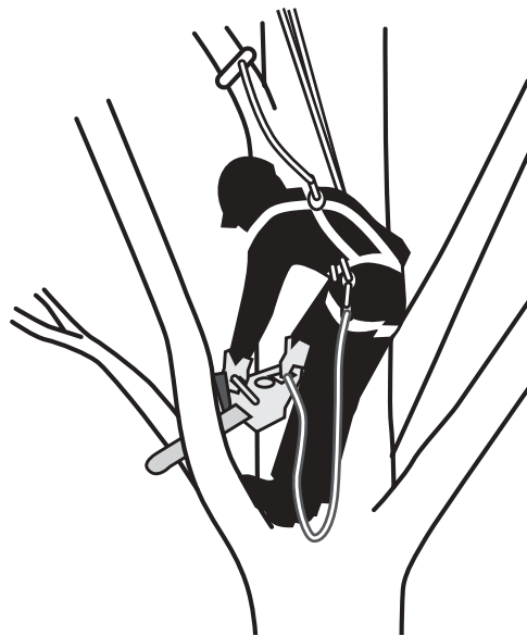
Above: When using a chainsaw in a tree, it should be attached to a lanyard that will allow the saw to drop below the climber's feet.
