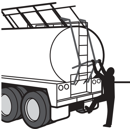
Above: Tanker showing fold down hand rails. Midrail and toe board are not shown for clarity of diagram.
